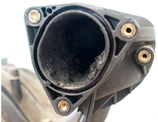
Picture 2: Intake manifold of a taxi after 150,000 km
