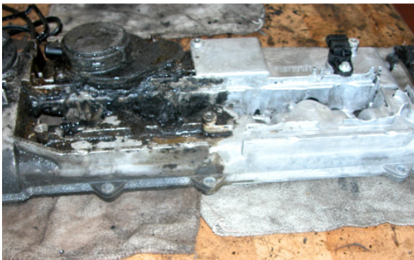
Removed valve cover. Left: untreated. Right: cleaned with Sealant Remover and engine wash.
