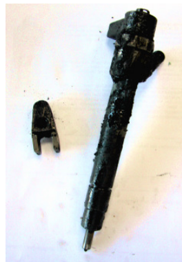
Removed injector with hard incrustation.
