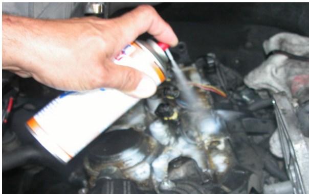
Spray all parts thoroughly with Sealant Remover and allow to work in.
